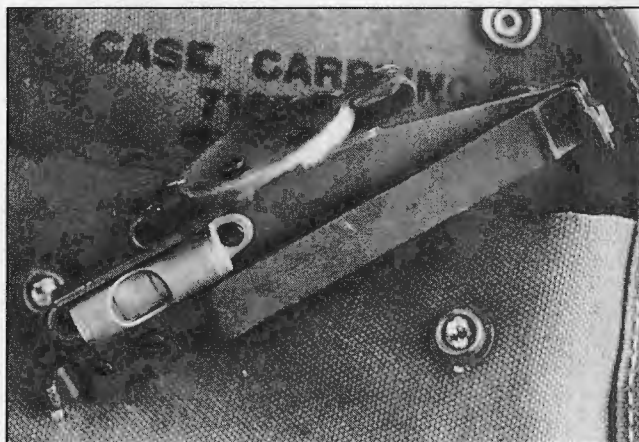
TOP: M14A1 muzzle compensator fits over flash suppressor and reduces felt recoil and muzzle climb.
